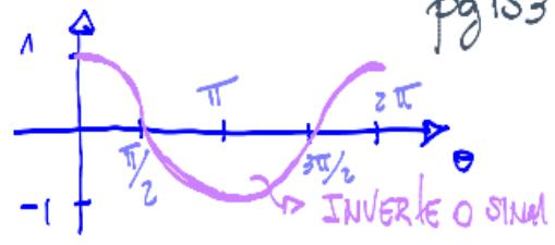
$$\bar{I}_{\text{ret}} = \langle I_{\text{ret}}(t) \rangle = \langle I_{\text{pico}} |\cos(\omega t)| \rangle = I_{\text{pico}} \langle \cos(\omega t) \rangle$$
